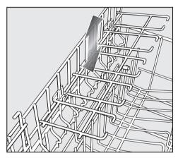
Slide the glass rack to the desired height until the catches click into place at the top and rest on the bottom.
